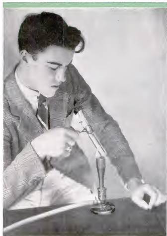
Bromine released by heating hydrogen bromide colors filter paper saturated with a reagent
